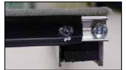
Reinstall the guide and assembly screw. Reassemble window and reinstall.
